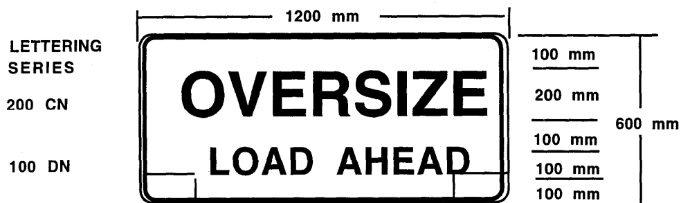
Warning sign that meets the minimum requirements for a warning sign on a pilot vehicle
