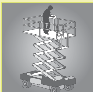
Figure 11: An example of a scissor-lift EWP. As with boom-type platforms, people should not climb onto or off the platform when it is in an elevated position.
