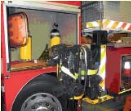
Breathing apparatus is stored in a side compartment. The breathing apparatus is fixed to an arm that can be extended out of the compartment. (Photo: R. Luke, thanks to SEM Fire & Rescue.)
