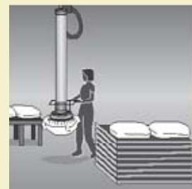
A vacuum operated lifting device can reduce the forces, awkward postures, and movements required to manually load products onto pallets.
