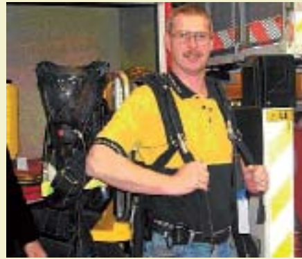
The person 'backs up' to the breathing apparatus. The apparatus is placed on shoulders without the awkward lifting that previously occurred. (Photo: R. Luke, thanks to SEM Fire & Rescue.)
