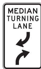
Median turning lane sign
