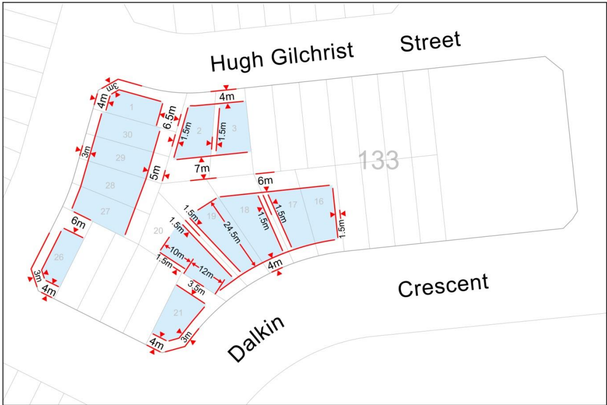
Figure 2c Detail of Maximum Building Zone - section 133
