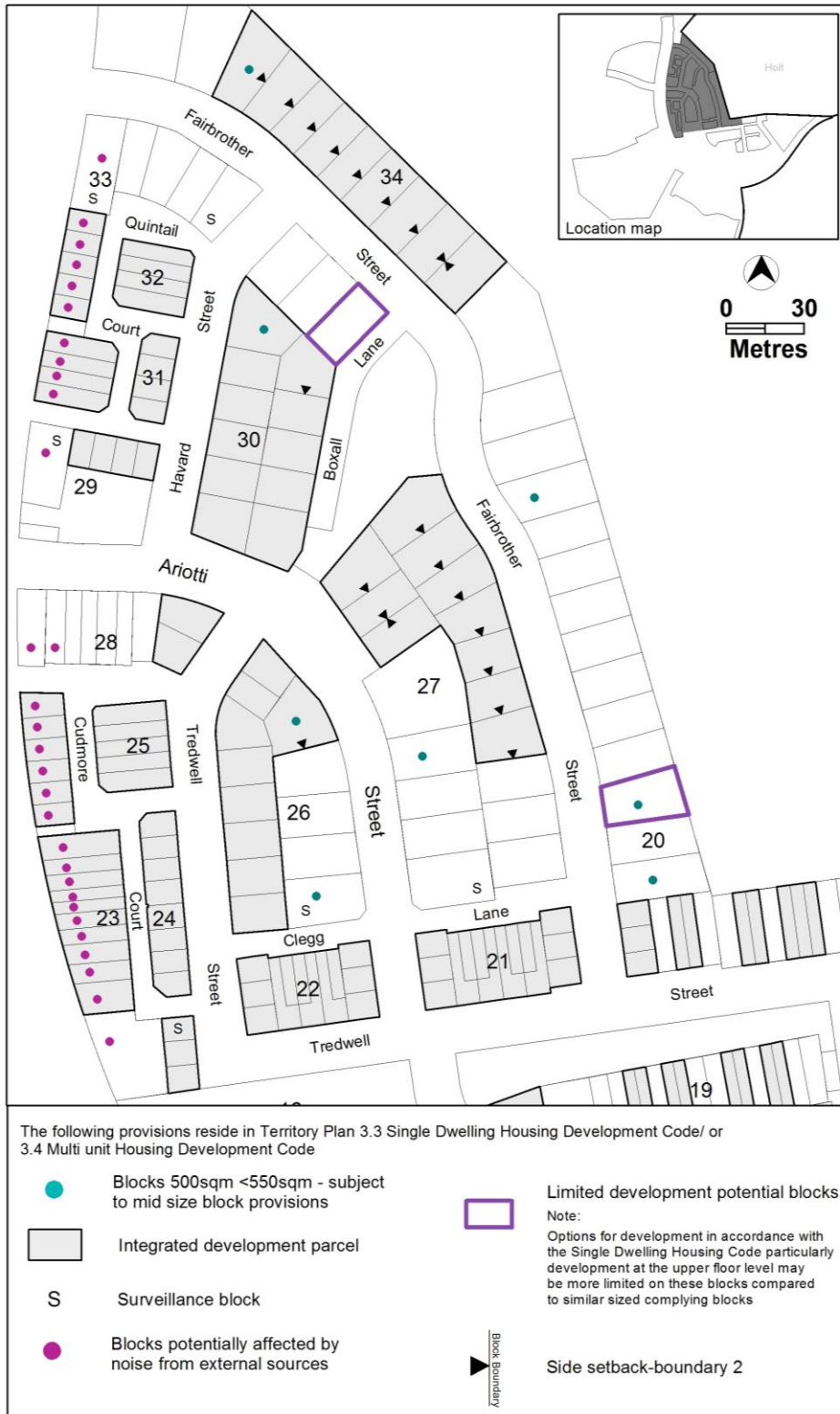
Figure 14 Strathnairn residential area ongoing provisions
