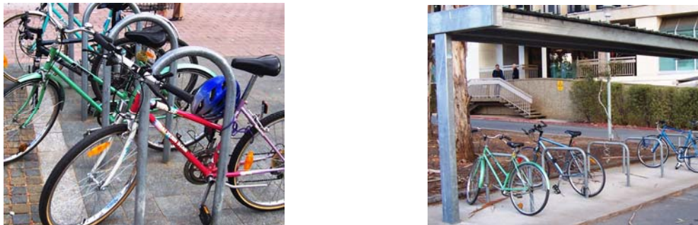
Figure 2 – Examples of Acceptable Bicycle Rail Parking Facilities
