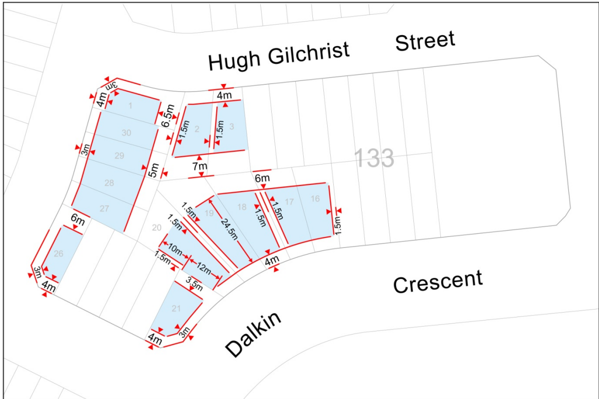
Figure 2c Detail of Maximum Building Zone - section 133
