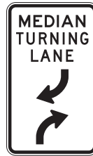
Median turning lane sign
