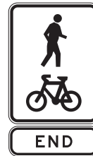
End shared path sign
