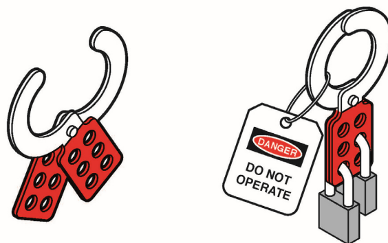
Figure 3: Example of tag and lockout with the padlocks of two workers.
