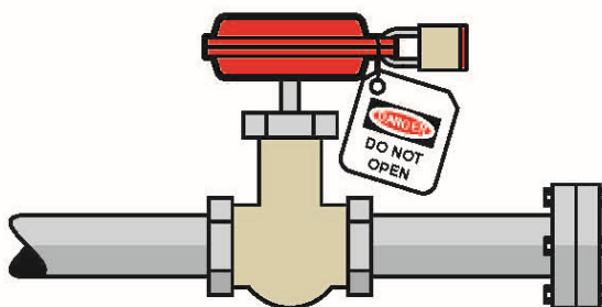
Figure 4: Open end of pipe capped. Nearest valve closed locked and tagged.
