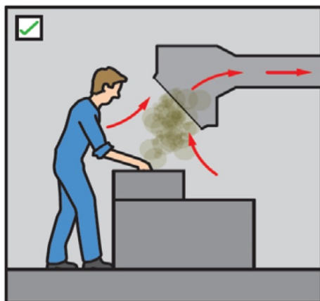
Diagram 4 Good design carries away contaminants from the operator's breathing zone
