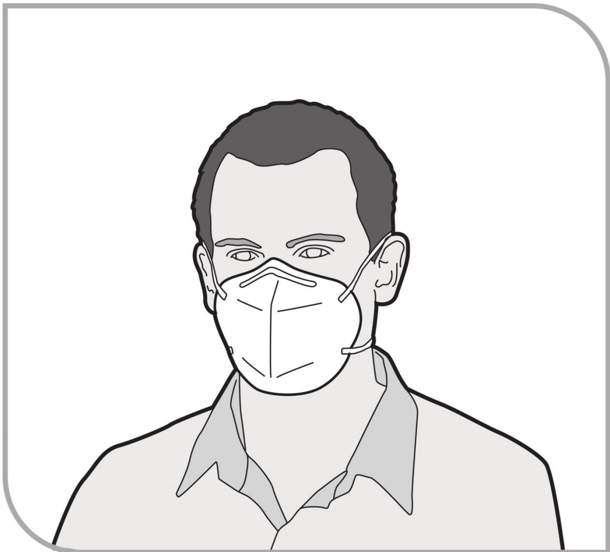
Figure 9 Disposable, half-face particulate respirator
