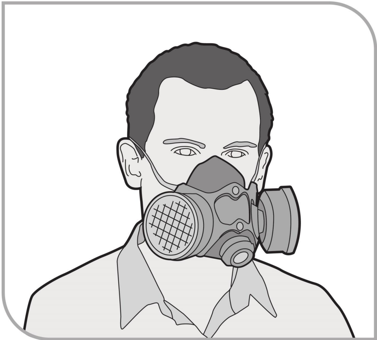
Figure 10 Half-face particulate filter (cartridge) respirator
