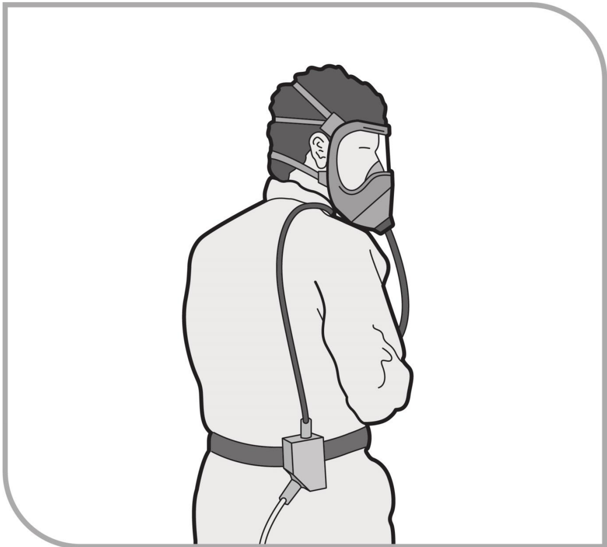
Figure 14 Full-face, positive pressure demand air-line respirator
