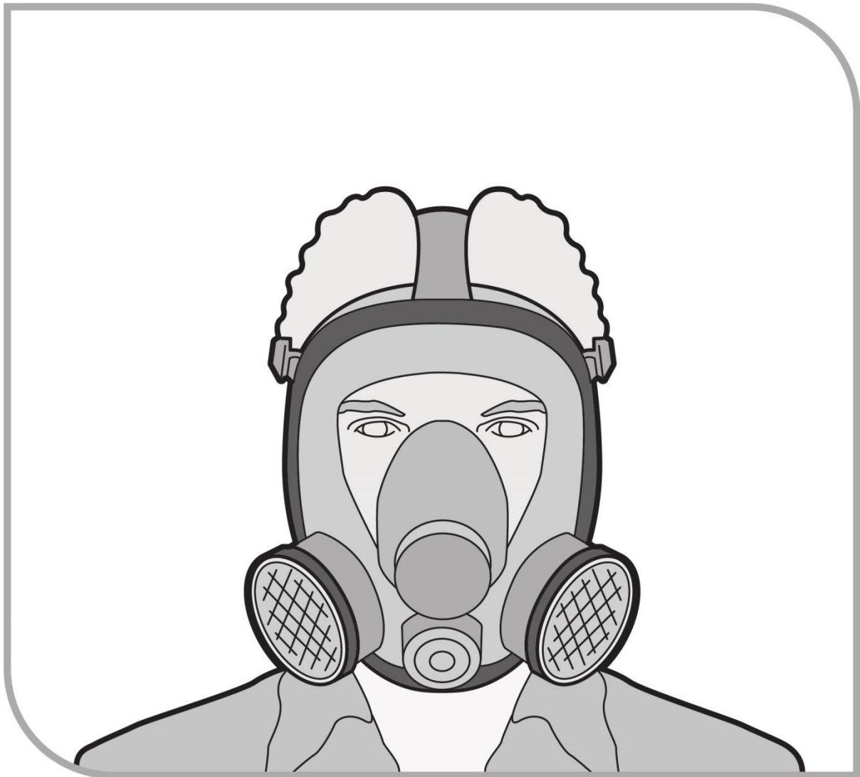
Figure 12 Full-face, particulate filter (cartridge) respirator
