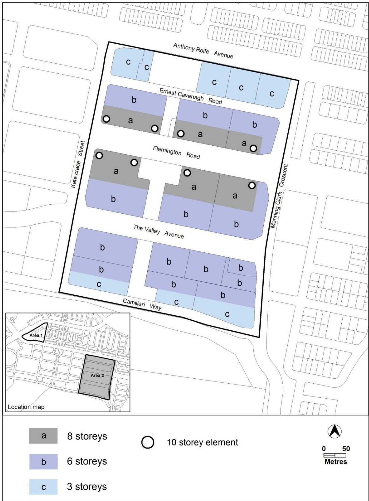
Figure 7 Gungahlin – Heights, Gungahlin Group Centre
