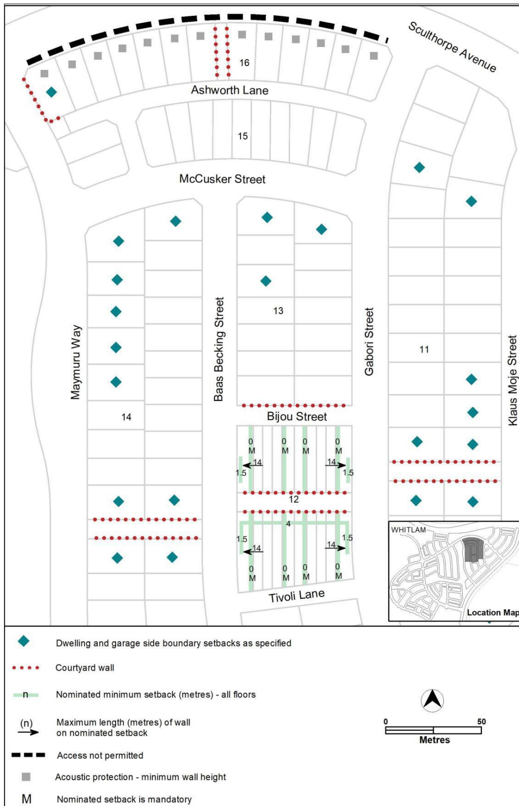
Figure 9 Whitlam – Development Requirements
