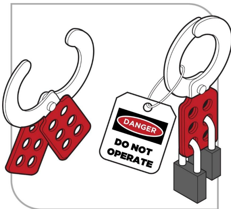
Figure 3 Example of tag and lockout with padlocks
