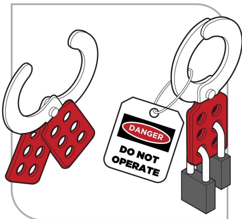
Figure 9 Example of lock-out with a tag and the padlocks of two workers
