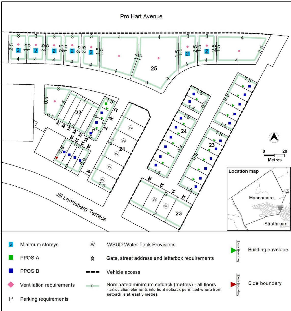
Figure 6 – Macnamara development requirements
