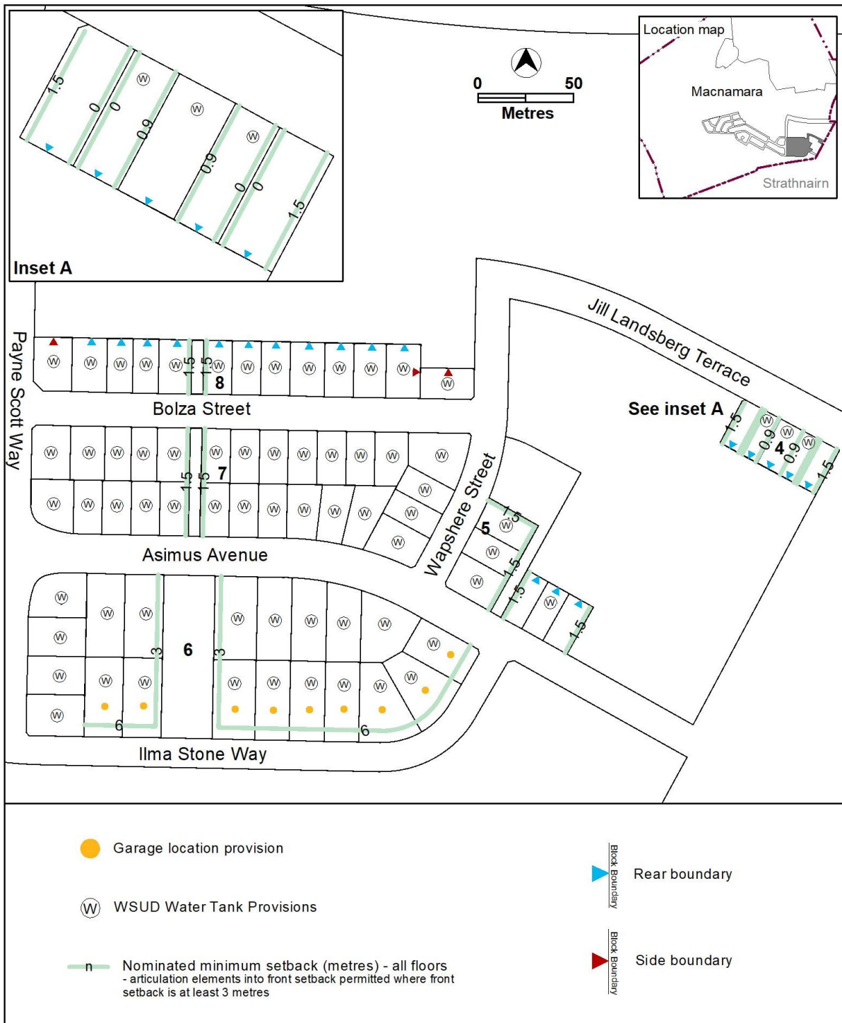
Figure 3 – Macnamara development requirements
