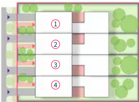
Figure 27: Terraces with individual parking from street. Individual parking from street can be appropriate on terraces with wide street frontages where dominance of garages on the frontage can be avoided. The site layout creates high amenity backyards for all dwellings.
