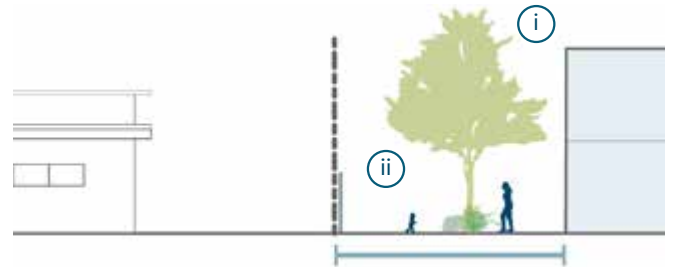
Figure 77: Rear setback: Rear setback zone to be used for larger consolidated garden areas and planted zones.
