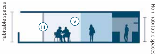
Figure 89: Determine ceiling heights in consideration of the depth and function of the space
