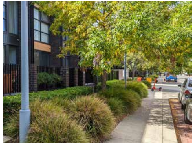
Photo 53: Fencing, planted areas, gates and slightly elevated ground floor level helps to balance privacy and street activation. Kingsborough Townhouses, ACT
