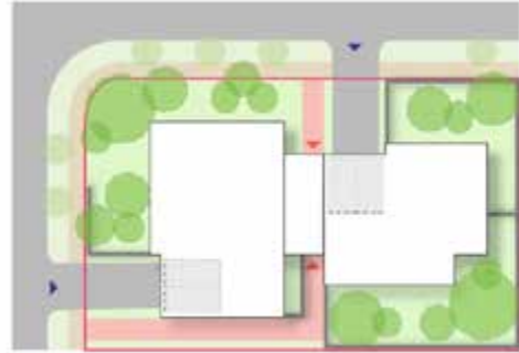
Figure 38: Corner block with individual car parking from street creates a high level of internal amenity and a suburban character.
