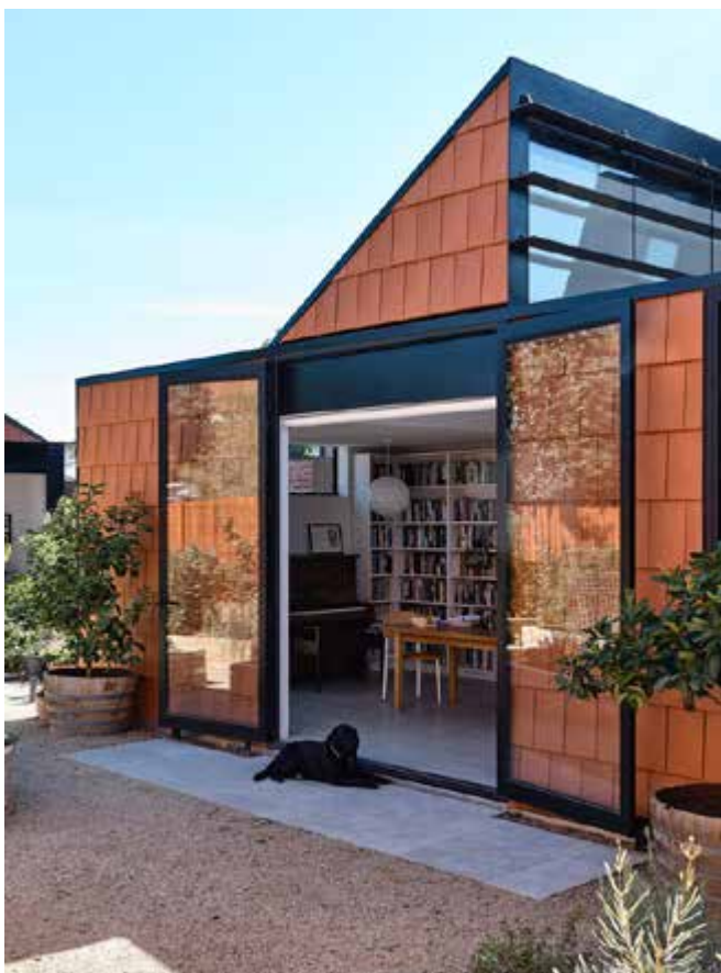
Figure 93: Introducing floor-to-ceiling windows with an increased ceiling height to the living space can provide daylight deep into the building while retaining outlook from upper levels.
