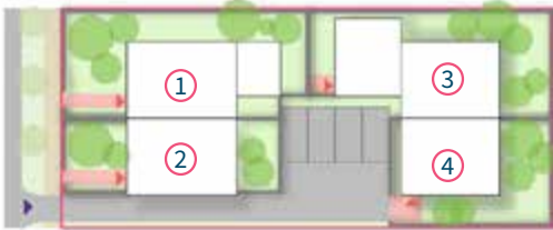
Figure 16: Shared parking in the centre of narrow sites maximises private open spaces.
