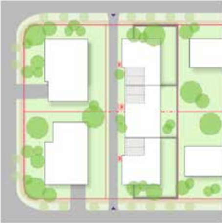
Figure 48: Mid section block consolidation example.
