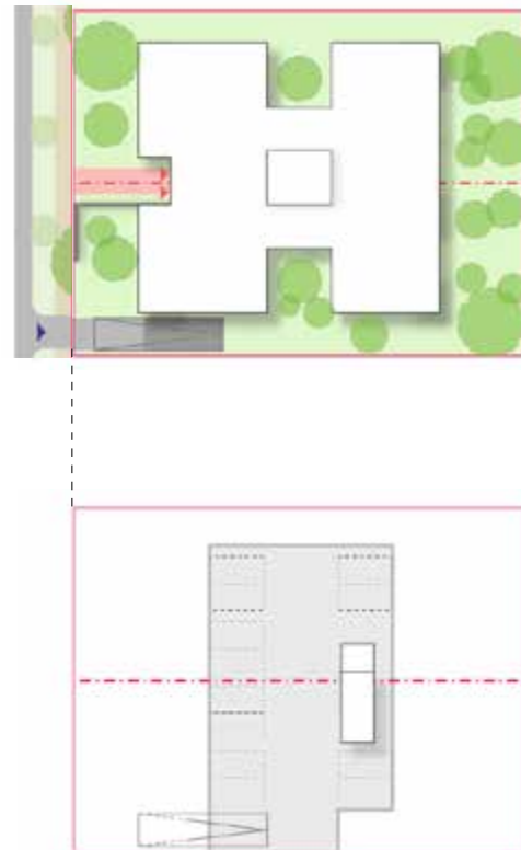
Figure 34: Apartments on consolidated block with shared basement parking from street. This layout maximises the opportunities for outlook and solar access for apartments.
