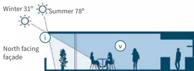
Figure 90: Design apartments with appropriate ceiling heights to ensure good access to daylight
