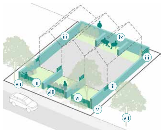
Figure 70: A range of fence heights between front, back, side and internal boundaries allow for a connection to the public realm and a strong sense of privacy for residents.
