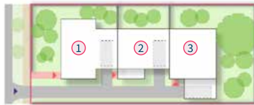
Figure 8: Attached tri-occupancy with parking access from primary road with parking within the building. Dwellings are placed to maximise private open space.
