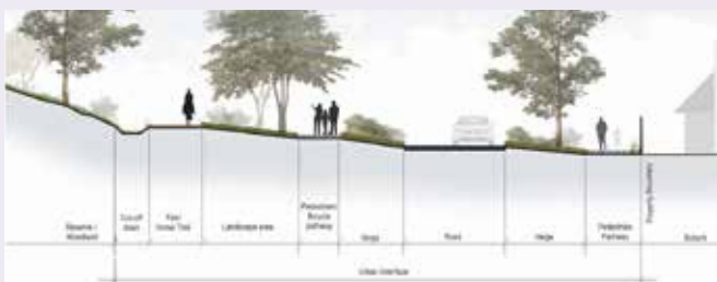
Figure 1 Typical cross-section for an urban interface zone where the adjoining natural asset is above the suburb. Source: Suburban Land Agency.
