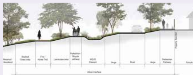
Figure 2 Typical cross-section for an urban interface zone where the adjoining natural asset is below the suburb. Source: Suburban Land Agency.
