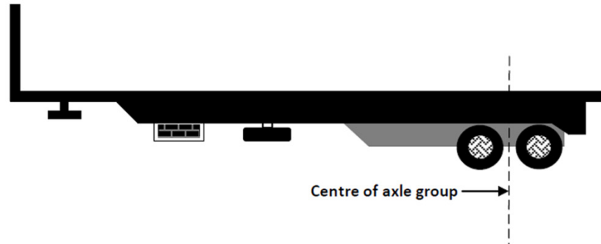
Centre-line of a tandem axle group fitted with an equal number of tyres on each axle
