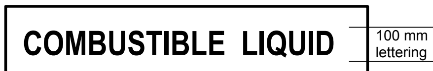
Figure 2.6—Placard for C1 combustible liquids
