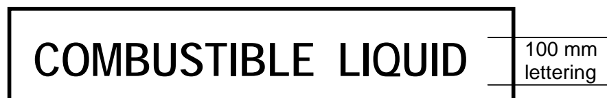
Figure 2.6—Placard for C1 combustible liquids
