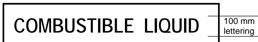
Figure 2.6—Placard for C1 combustible liquids
