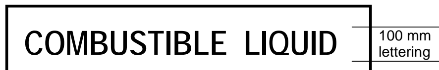
Figure 2.6—Placard for C1 combustible liquids
