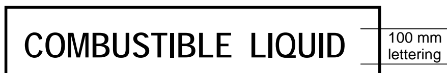
Figure 2.6—Placard for C1 combustible liquids
