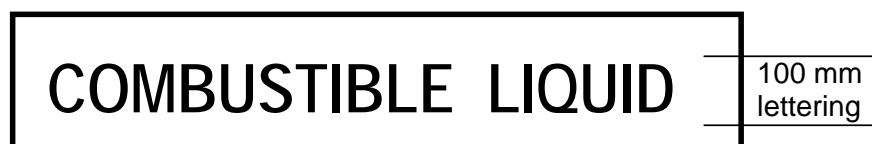
Figure 2.6—Placard for C1 combustible liquids
