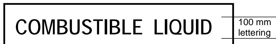
Figure 2.6—Placard for C1 combustible liquids
