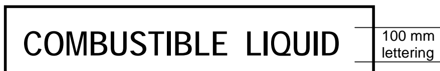
Figure 2.6—Placard for C1 combustible liquids
