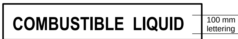
Figure 13.5 Placard for flammable liquid category 4
