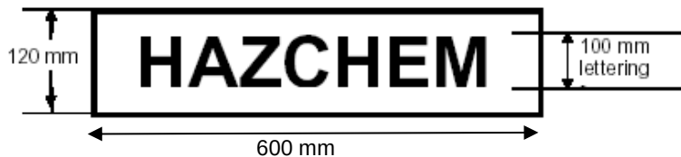
Figure 13.1 Form and dimensions of outer warning placard
