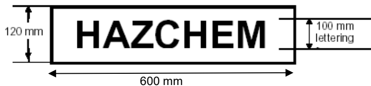
Figure 13.1 Form and dimensions of outer warning placard
