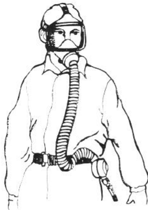
FULL-FACE, POSITIVE PRESSURE DEMAND AIRLINE RESPIRATOR
